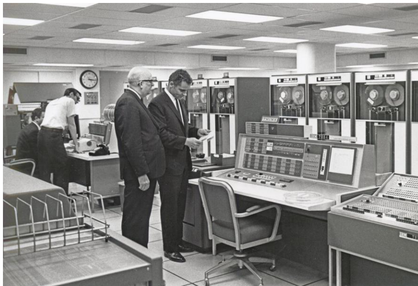
The Medical Centre's IBM 7904 mainframe computer system, circa 1969. The entire computer once took up almost half a building, the other half was the air conditioning
